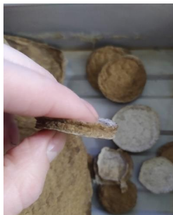
Fig. 4. Material with added glycerine and potato starch
