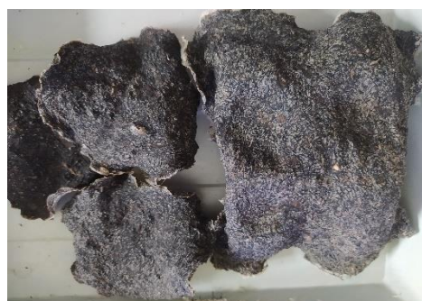
Fig. 5. Material with added glycerine, potato starch and seaweed particles
